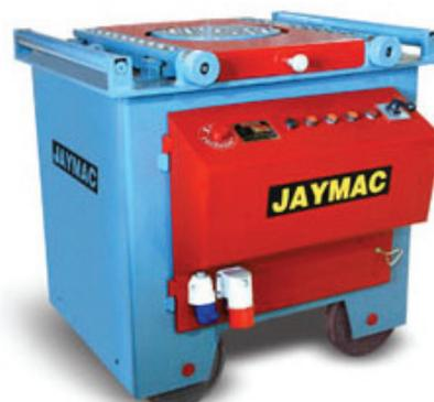
effective machine, used for bending reinforcement bars and various forms of round bars.
